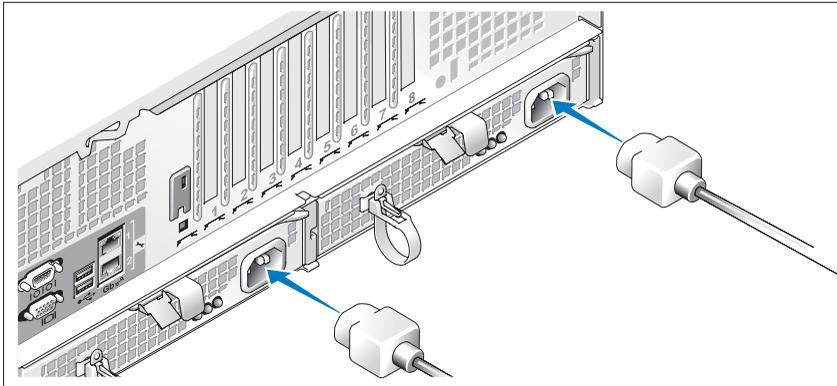
Connect the monitor's power cable to the monitor (optional). Connect the system's power cables to the system.
